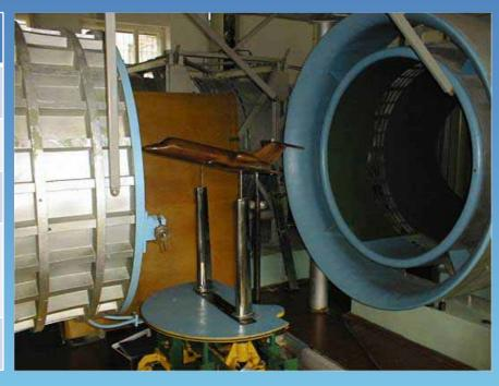
• Scale Model of UAV in Working Section of Wind Tunnel *T-4*
